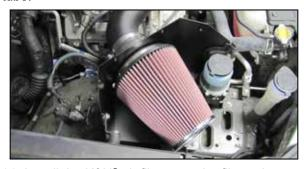
31. Install the K&N® air filter onto the filter adapter and secure with the provided hose clamp.
