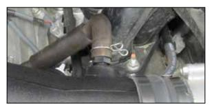
29. Connect the crank case vent line to the 5/8 vent fitting and secure with the factory spring clamp.
