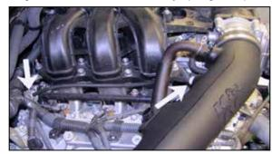
30. Connect the provided fuel pressure vent line to the fuel pressure regulator and then connect the open end to the 3/16 vent fitting in the K&N® intake tube.
