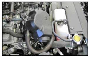
11a. Lift up the air injection pump, disconnect the electrical connection and then set the air injection pump over to side.
