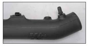
26. Install the 5/8 vent fitting into the K&N® intake tube as shown.
