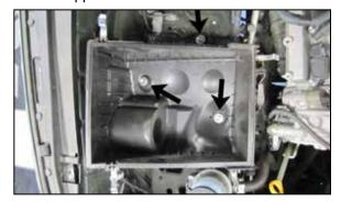
9. Loosen and remove the three bolts securing the lower air box and then remove the lower air box from the vehicle.
