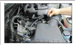
3. Disconnect the mass air sensor electrical connection and then unhook the wiring harness from the air box.
