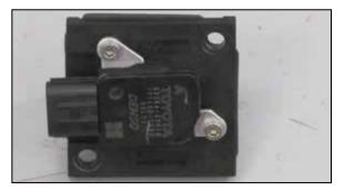
24. Install the mass air sensor into the K&N® mass air sensor adapter and secure with the provided hardware
