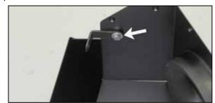
16. Install the provided mounting bracket (08022) onto the heat shield and secure with the provided hardware.
