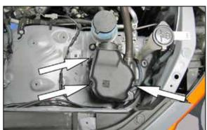
11. On models with the Air injection pump located in front of the air box next to the Power steering reservoir, remove the three bolts securing the pump to the inner fender.
