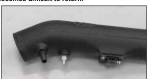
27. Install the 3/16 vent fitting into the K&N® intake
