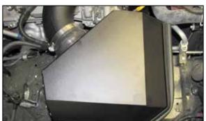
33. Install the heat shield cover onto the heat shield and secure with the provided hardware.
