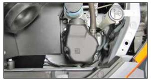
19a. Install the air injection pump onto the heat shield and forward rubber mounted stud and then secure with the provided hardware. Reconnect the air injection pump electrical connection.
