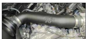
28. Install the K&N® intake tube into hump hose at the filter adapter and then into the silicone hose at the throttle body, align the tube for proper fit and then tighten the hose clamps.
