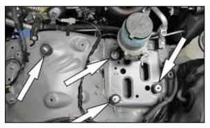
12. Install the four rubber mounted studs into the factory air box and P/S reservoir as shown.
