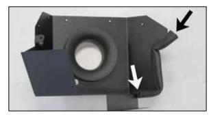
18. Install the 10.5" long piece onto the heat shield as shown.
