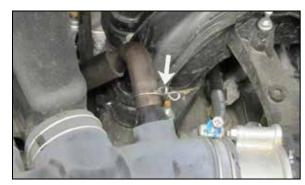
5. Disconnect the crank case vent hose from the stock intake tube.
