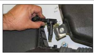
23. Remove the screws which secure the mass air sensor to the factory air box and then remove the mass air sensor from the air box.
