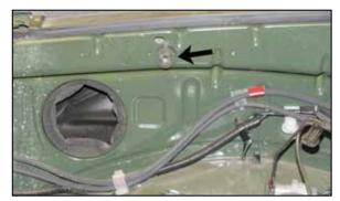
13. Install the 6mm rubber mounted stud into the inner fender location shown.
