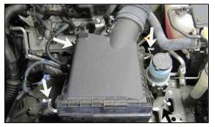
8. Release the four clips which secure the upper air box to the lower air box and then remove the intake tube and upper air box from the vehicle.
