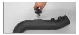
25. Install the mass air sensor assembly into the K&N® intake tube and secure with the provided hardware.
